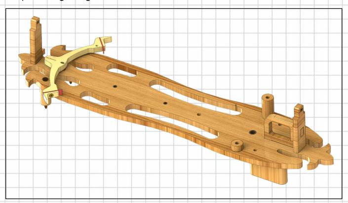
The Escapement Arm needs to be assembled and fitted with the Pallets and the Pallet clamps and laid in position at the top of the Back Frame. The shaft that this attaches to is on the Pendulum assembly and so will be fitted later.
