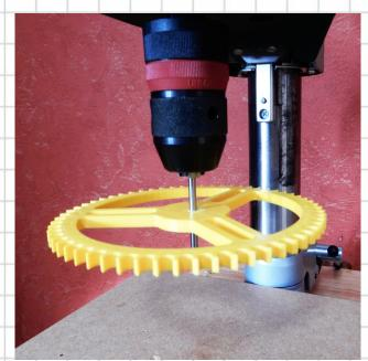
The Gear shown above is required to be assembled with care to ensure the shaft fits square to the gear. I recommend you use a drill press to do this as I have done, as it ensures that the gears are mounted square to the shaft.
