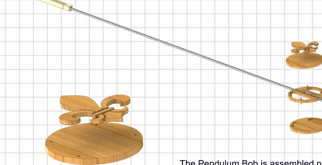
The Pendulum Bob is assembled next the 3 disks the Top Centre and Bottom are all pinned together with the 4 short pins. Before actually fitting the top disk you need to press the lock piece into its position and and fill the pockets with ball Ø8 or 9 mm Ball bearings.
