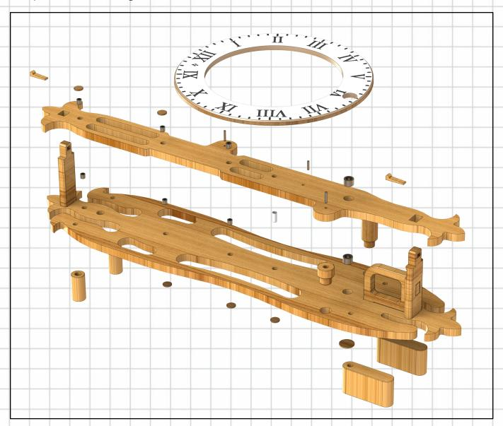
First task is to assemble all of the frame parts as shown in the picture above. This is to include all of the bearings Blanking caps being glued to the outside of the shaft holes in both frames. This includes the the short bearing sleeve in the centre of the front frame which is used instead of a bearing to give addition support to its shaft which is held on one side only.
