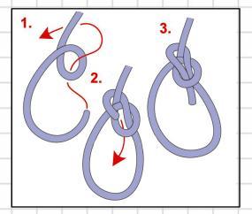
I always use a Bow Line Knot on the end of the cord holding the driving weight of a clock, it is one of the most useful knots you can know. The Bowline forms a secure loop that will not jam and is easy to tie and untie. The Bowline is most commonly used for forming a fixed loop, large or small at the end of a line. Tried and tested over centuries, this knot is reliable, strong and stable. Even after severe tension is applied it is easy to untie.
