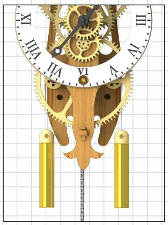
First glue the Weight Tops to the weight using superglue, now position the loop of the knot into the slot at the top of the weight and push the Pin through the cross hole and let go, the clock is ready to run
