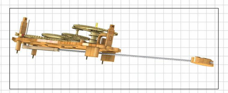
Fit the pendulum simply by pushing the two shafts at the top through the bearing at the top and into the two holes in the Escapement arm. The long Pivot shaft should be a Press fit in the Escapement arm. The shorter shaft is to make sure the Pendulum and the Escapement Arm move together.
