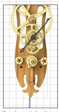
If you have not done it already then attach the two cords to their respective drums and then wrap them over their pulleys in the manner shown above. The weights need to turn the drum anti clockwise so they need to be pulling on opposite sides of the drum to ensure that is done, otherwise you will get no movement at all.
