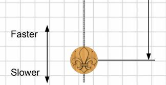
Initially set the Pendulum Bob so the distance to the pendulum pivot is 1050mm (41.5 inches).
