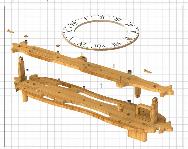
The two frame spacers and and the wall spacers on the underside are the first to be glued into place.
