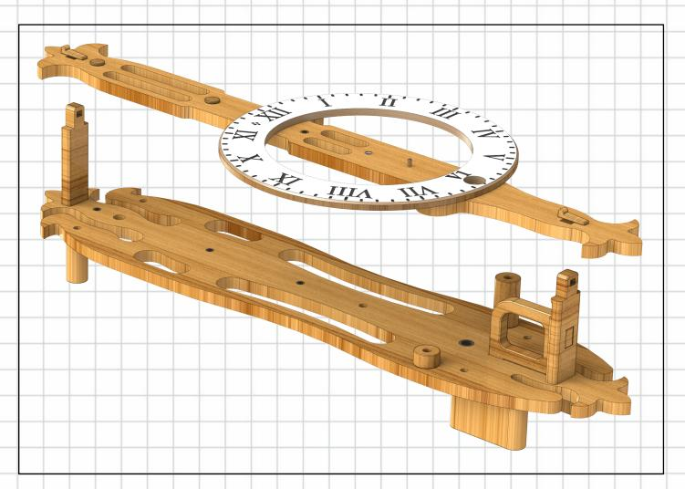
Next all the bearings are press fitted into the inside faces of the front and Back frames plus fitting the 3 short pins in the outside face of the Front Frame, two that hold the dial in place and one inside them for the Hour gear pivot. The Dial is then fitted to the pins and glued to the front face.
