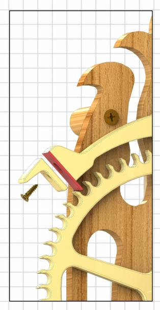
For the clock to run correctly the Escapement should be set so that the swing of the pendulum moves the pallets in and out of engagement with the teeth evenly.
